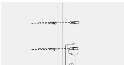
If the wall of the house is not made of wood, you should drill dowel holes 5 mm (0.19 in) in diameter in the wall according to the drilling template and then place the dowels provided into the boreholes.
