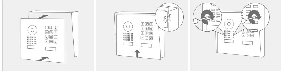
While turning the screws clockwise, press the front panel firmly onto the housing until the screws are tightened.
