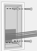
Please make sure that the outer frame of the flush-mounted housing rests on the outside of the wall and that the edge of the flush-mounted housing is sealed all around against moisture from the outside.
