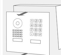
Pull the front panel with attached Main Electrical Unit out of the mounting housing (backbox).
