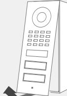
Pull the front panel with attached Main Electrical Unit out of the mounting housing (backbox).
