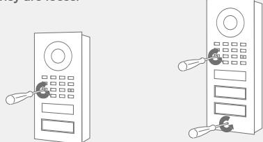
Turn the safety screws counter-clockwise until they are loose.
