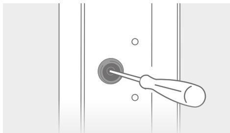
Pierce through the middle of the rubber seal using a screwdriver.
